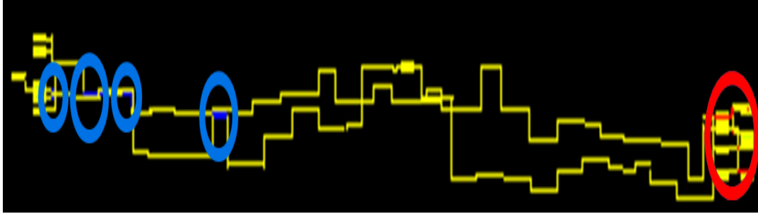
Figure 4-1 An example of a bridge fault
